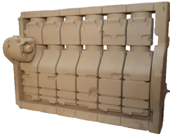
6 CYL. BLOCK Core-Assembly Weight: 169 kg
