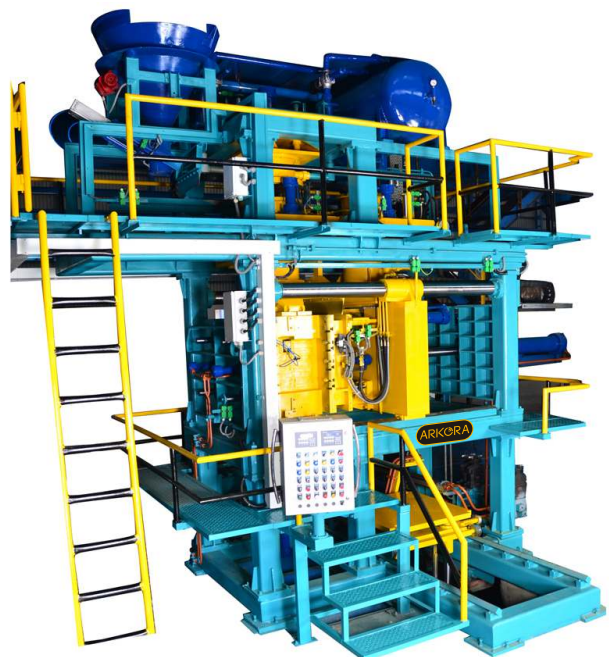
Cold Box 120 Ltr Vertical Parting (with tilting arrangement )
