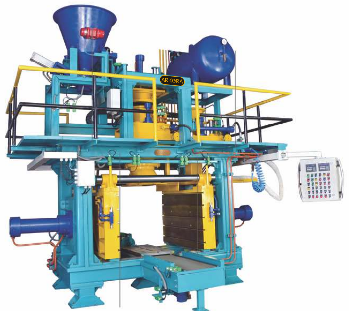
Cold Box 80 ltr Vertical Parting (with both halves moving)
