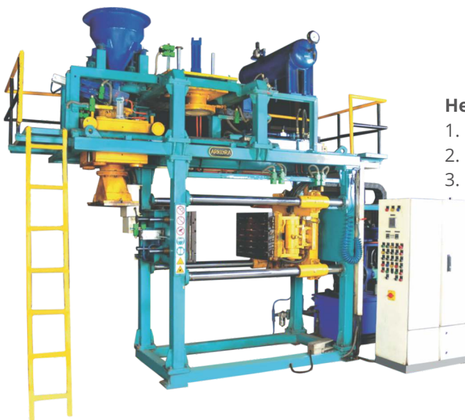
Shell Shooter 10 Itr Vertical Parting (with swing arrangement)
