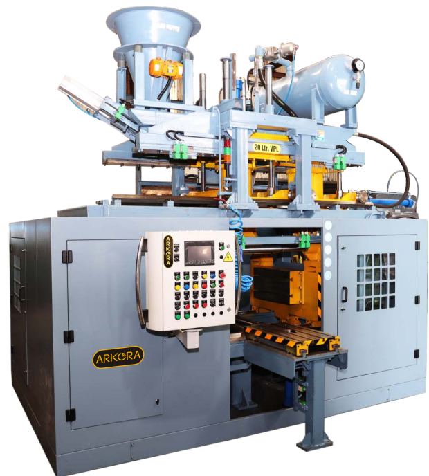
Cold Box 20 Ltr Vertical Parting (with both halves moving)
