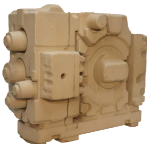
GEAR BOX HOUSING Core Weight: 103 kg+ 48 kg Core Assembly Weight: 151 kg
